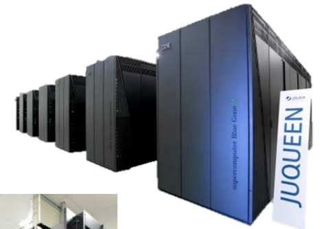
JUQUEEN IBM Blue Gene/Q 5.9 PFlop/s in 2.3 MW
